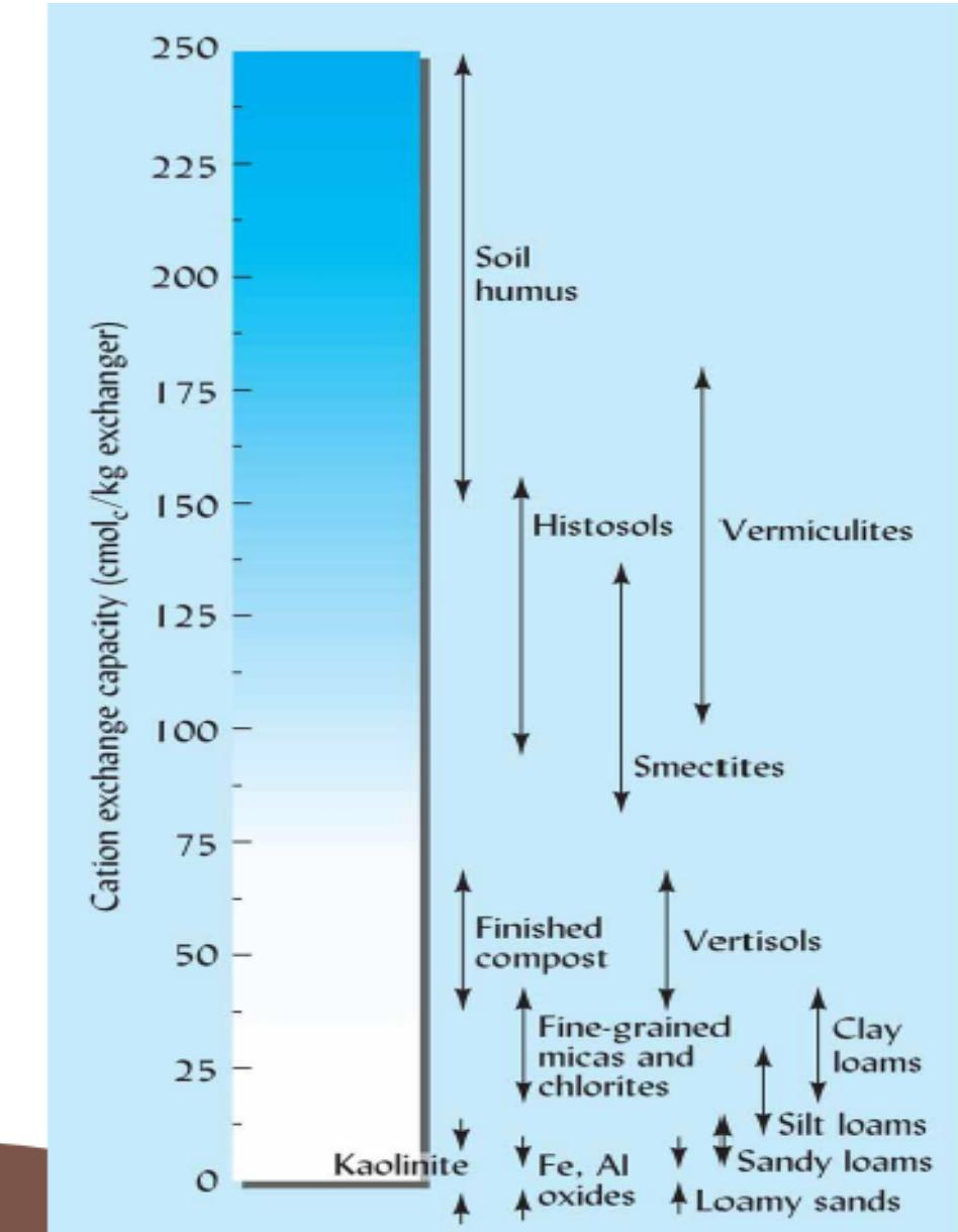
Ranges in the cation exchange capacities (at pH 7) that are typical of a variety of soils and soil materials.
